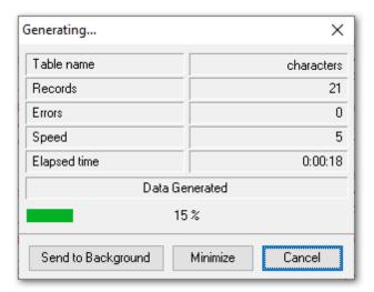
Use the **Send to background** button to run the process in the background mode, the **Minimize** button to minimize the application to Windows Task bar, or the **Cancel** button to stop the generation process.
