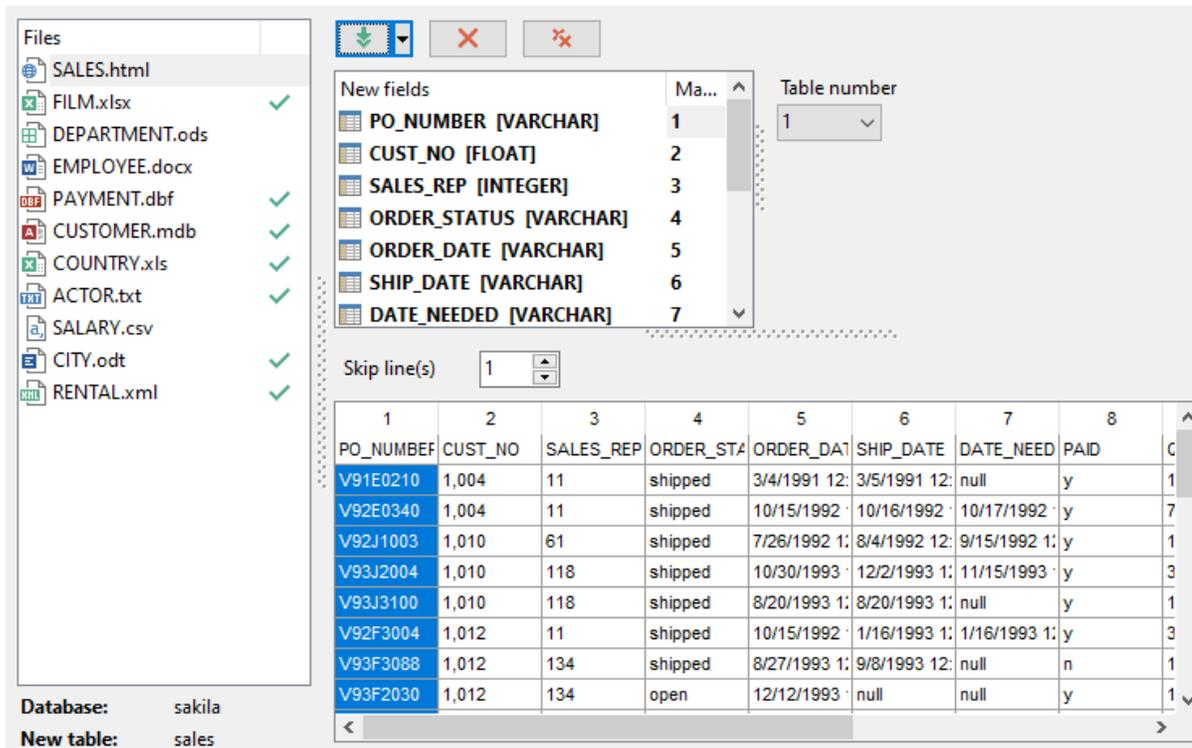
The screenshot shows the data import interface. On the left is a file list with various documents. In the center, there are controls for field mapping, including a 'New fields' list, a 'Table number' dropdown, and a 'Skip line(s)' input. On the right, a data preview table is shown with columns 1 through 8 and a 'C' column for column numbers.
